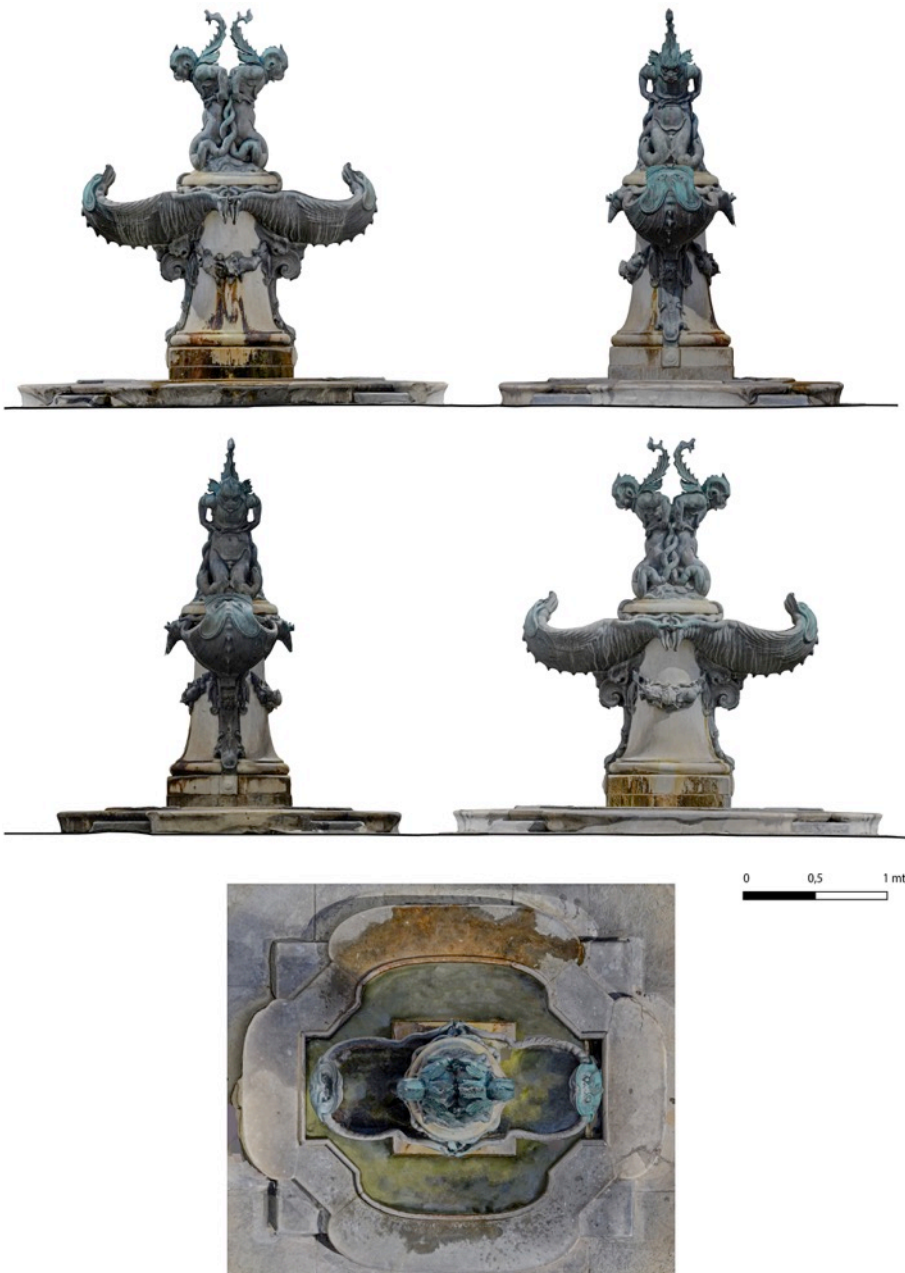
Figure 7 – Orthographic views of the digital 3D model of the western fountain in Florence.
